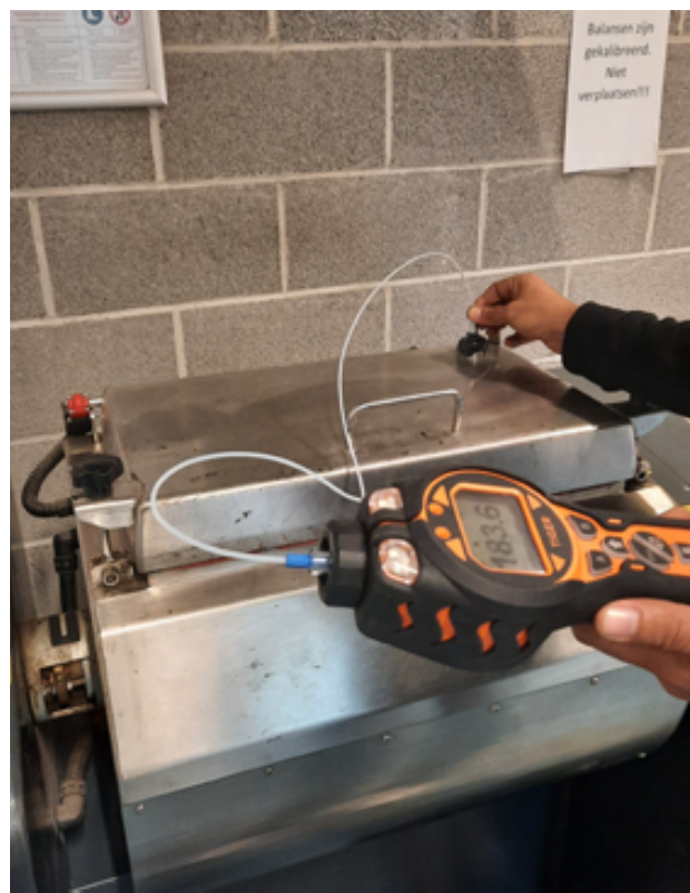
Ion Tiger VOC gas detector using photoionisation (pid). Image courtesy of J. Blom.
