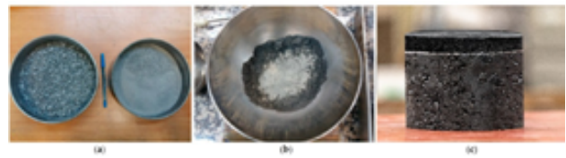
Microsurfacing production and specimen preparation: (a) aggregate fraction separation, (b) mixing phase (addition of cement), (c) double-layered specimen ready for testing. Image courtesy of C. Sangiorgi.
