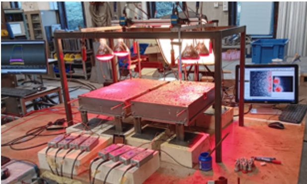
Acoustic Monitoring of Internal Curing of Fresh Concrete With Superabsorbent Polymers under Drying Conditions ©Mechanics of Materials and Constructions Department (MEMC) of Vrije Universiteit Brussel (VUB). Funding from Fonds Wetenschappelijk Onderzoek - Vlaanderen, FWO in cooperation with Magnel-Vandepitte Laboratory, Ghent University (UGent)
