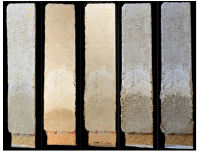
Deterioration of a 2-layer composite, comprising of natural stone and CEB, induced by continuous partial immersion in water ©Ledra & Building Materials Laboratory, University of Cyprus
