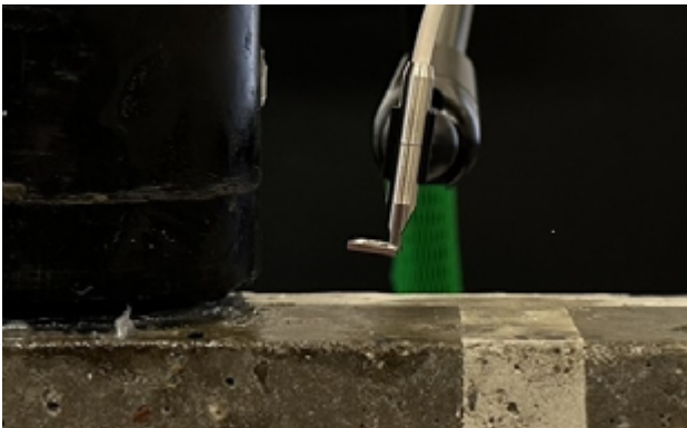
Air-coupled ultrasonic monitoring of concrete and difference in wave velocity dispersion curve between healthy and chemically attacked concrete, MEMC-Vrije Universiteit Brussel, FWO © TC 269-IAM
