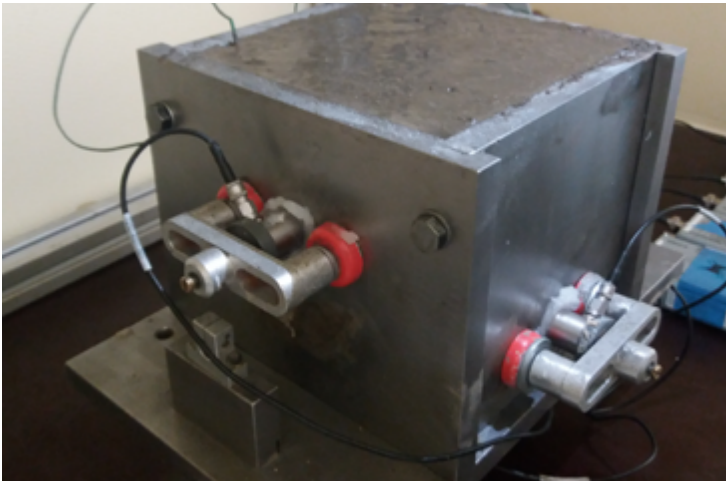
Fresh Concrete monitoring by acoustic emission sensors and real time localization of internal curing activity due to SAPs ©MEMC-Vrije Universiteit Brussel, FWO, TC 269-IAM
