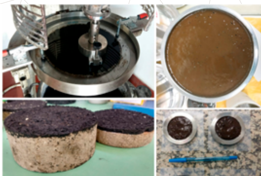
Tests on slurry surfacings carried out within the TG2 interlaboratory test. Image courtesy of C. Sangiorgi, C. Raab and J. Oliveira.
