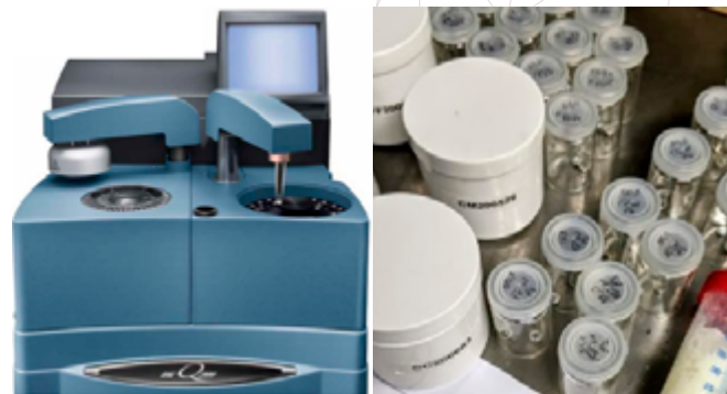
Heat storage capacity of PCM using dynamic DSC tests. Picture courtesy of A. Caggiano.
