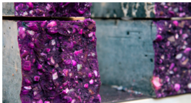
Alkali-activated slag concrete specimens after spraying with phenolphthalein to determine their initial carbonation depths. Image courtesy of BAM.
