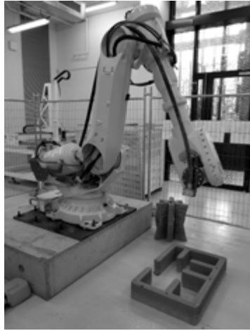
3D concrete printing laboratory Swinburne University of Technology, Melbourne, Australia @Jay Sanjayan
