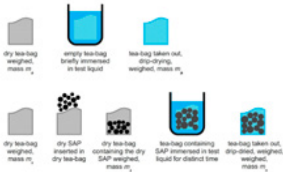
Tea-bag method to test SAP absorption. Materials and Structures (2018) 51:116.
