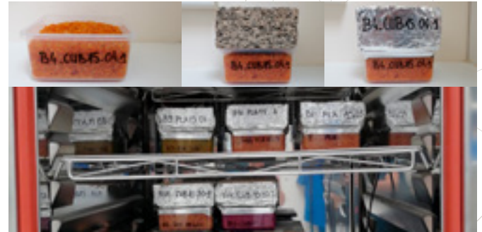
Measurement of Water Vapor Permeability of Hemp concrete at LGCGM / Université de Rennes 1 (France): cup assembly and test. Courtesy of F. Collet.
