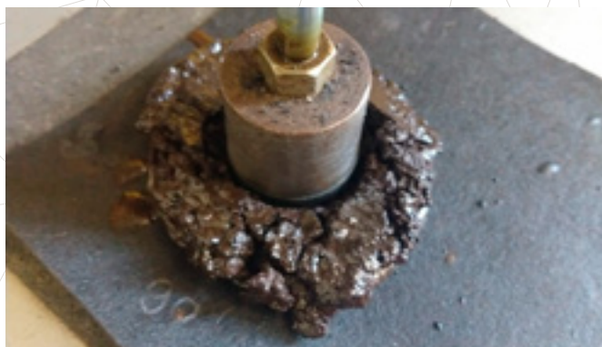
Cohesion test on bituminous slurry surfacing. Courtesy of C. Sangiorgi.
