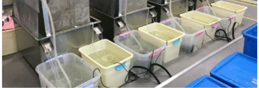
Room Test for reinforced concrete durability under combined role of sulphate and chloride. Courtesy of Mu Song.
