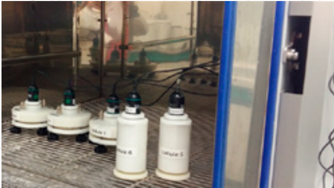
Diffusion cell in RH chamber. Courtesy of LafargeHolcim.
