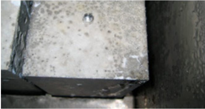
Accelerated concrete prism testing at 60°C – RILEM-AAR-11. Courtesy of B. J. Wigum.
