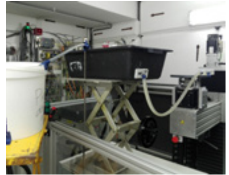
Determination of liquid permeability by CT scanner at Gent University. Courtesy of H. Derluyn.
