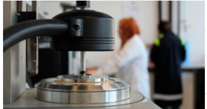
Bitumen sample ready to be tested in a dynamic shear rheometer (DSR). Courtesy of B. Hofko.
