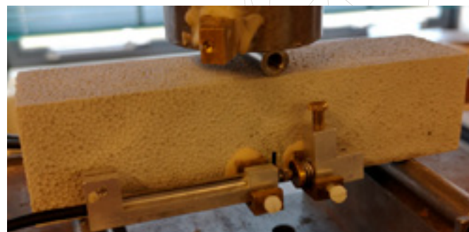
Notched sample of AAM. Courtesy of TC MPA.
