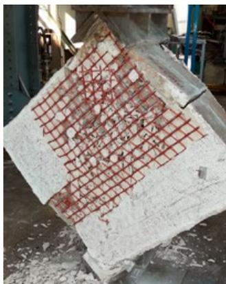
Crack pattern of a similar wall, though bigger, captured using the digital image correlation (DIC) method
