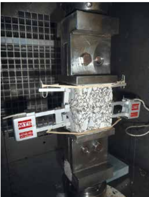
The EBADE test is a strain sweep test developed at the Road Research Laboratory of the UPC that provides information about the fatigue cracking resistance of asphalt mixtures, reducing considerable the testing time with respect to the conventional test procedures employed to that purpose. Credits: Ramón Botella Nieto
