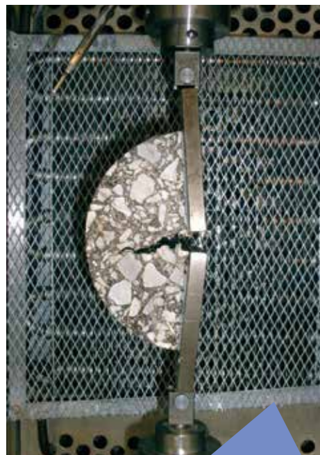
The Fenix test is a monotonic test developed at the Road Research Laboratory of the UPC that characterizes the cracking resistance of asphalt mixtures. Credits: Ramón Botella Nieto
