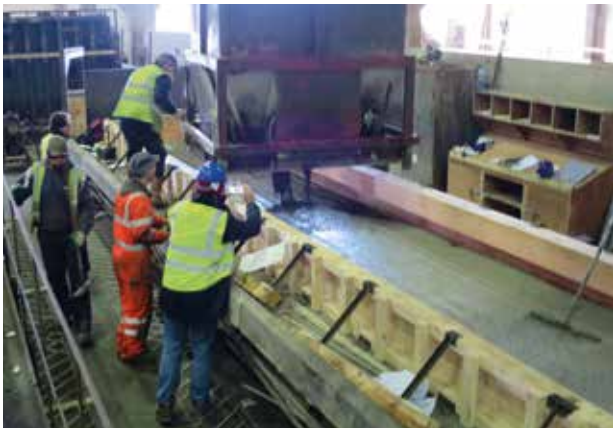
Testing 10-m Precast Fibre Reinforced Self-Compacting Concrete (FRSCC) slab pre-stressed with Basalt Fibre Reinforced Polymer Bars (BFRP): FP7-IAPP-Eurocrete Project 2013-2017. Credits: Mohammed Sonebi
