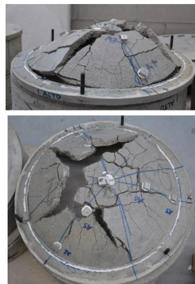
a) Impact on protective foams; b) impact on HPFRC slabs [6].
