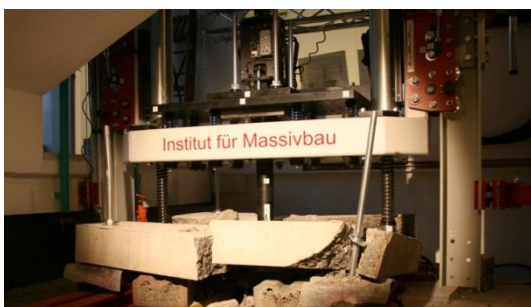
View of the drop tower setup field with damaged sample
