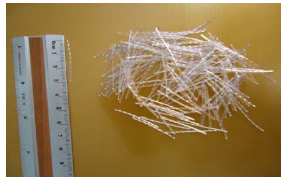
Fig. 2 : Picture of Virgin PP fibres used in the study.
