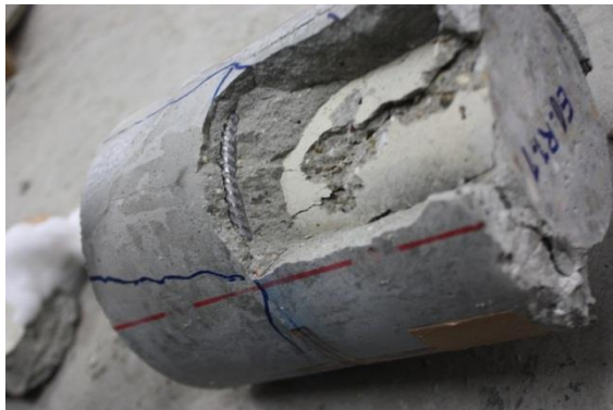
c) specimens having one stirrup 1φ6 (0.56%)
