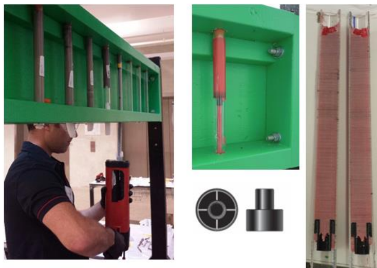
Figure 16. Overhead injection with a piston plug, tube is sliced after curing time is complete to check for voids.
