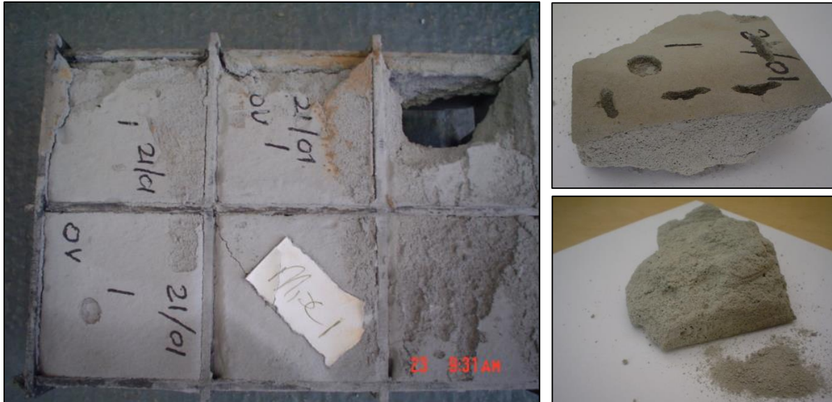
Figure 2. Damaged low density AAFC.
