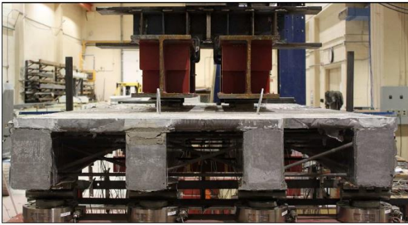
Figure 1. Dimensions and photograph of quarter-scale hybrid steel-free multi-girder bridge deck system.
