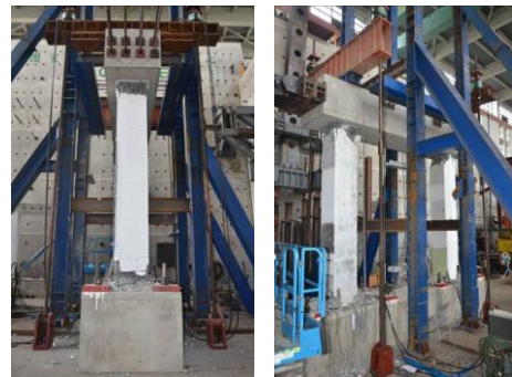
Figure 14. Push-over test setup.
