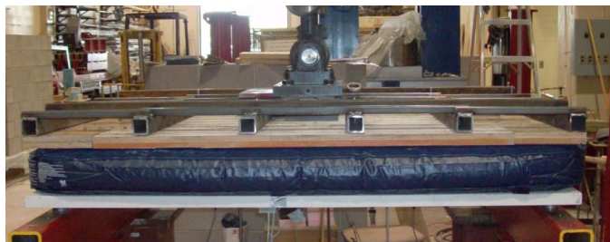
Figure 7. Use of an air mattress to provide uniform pressure
