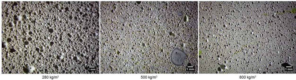
Figure 3. Pore sizes in foam concrete of various densities.
