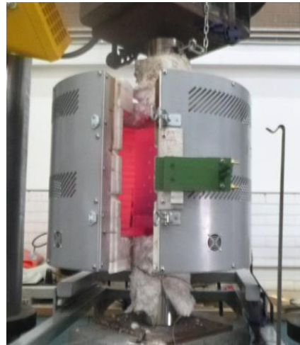
(b) Furnace and loading furnace during heating (furnace door was opened for photographic purpose only)
