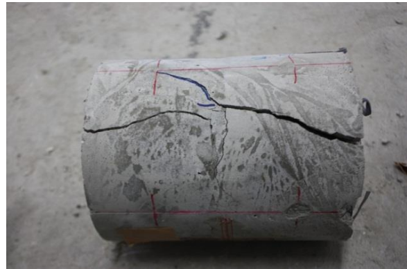
c) specimens having one stirrup 1φ6 (0.56%)
