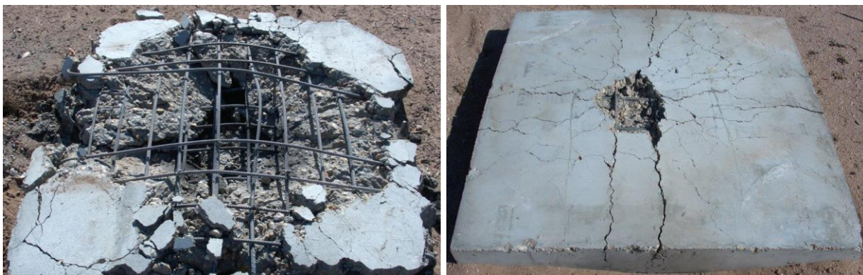
(a) Control 2 Layers of 10 mm Bar at 100 mm
