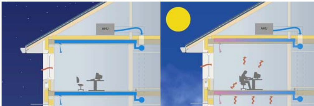
Figure 4. Example of the use of thermal mass in decks during summer: a) night and b) day
