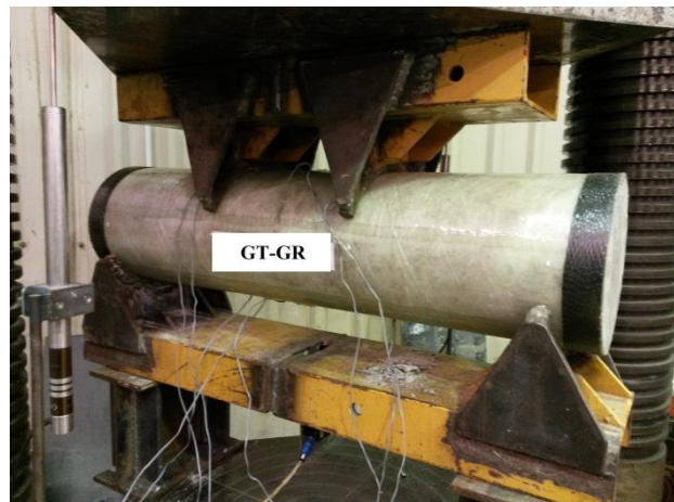
Figure 1. Flexural testing arrangement used in this study
