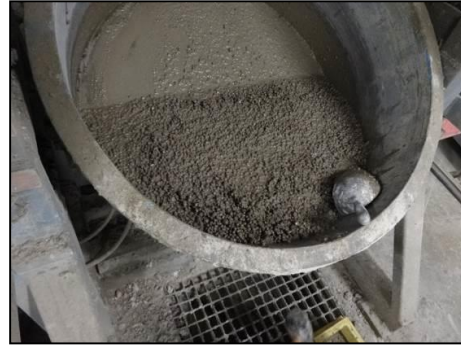
Figure 9. GP fresh concrete Recipe 1 (cone 26 cm). Figure 10. GP fresh concrete Recipe 2 (cone 27 cm).
