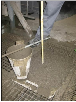
Figure 9. GP fresh concrete Recipe 1 (cone 26 cm). Figure 10. GP fresh concrete Recipe 2 (cone 27 cm).
