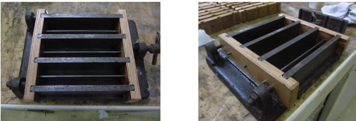
Figure 5. Adjusted form for manufacture of test specimens with holes for placing and fixing steel reinforcement
