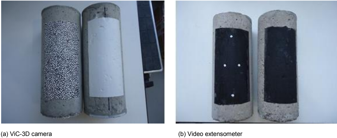
Figure 4. Surface preparation for strain measurement
