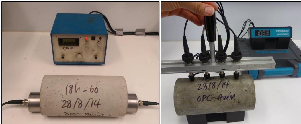
Figure 3. Pulse velocity (left) and surface resistivity (right) tests
