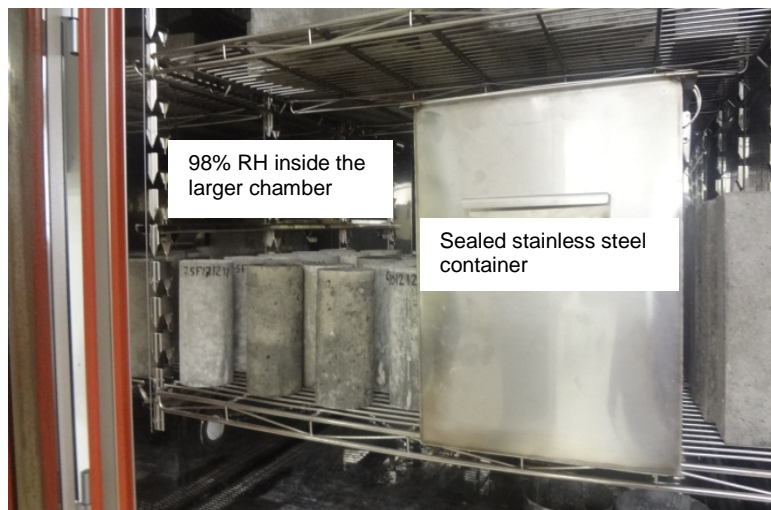
Figure 1. Chamber where samples were stored at specified temperature and humidity.
