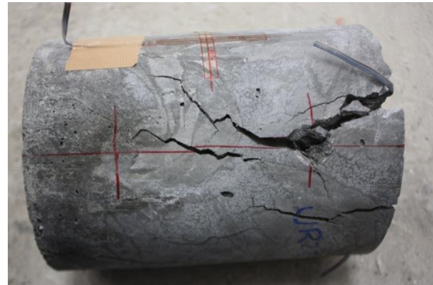
d) specimens having three stirrups 3φ6 (1.7%)
