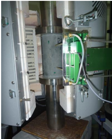
(a) Arrangement of furnace with extensometer.
