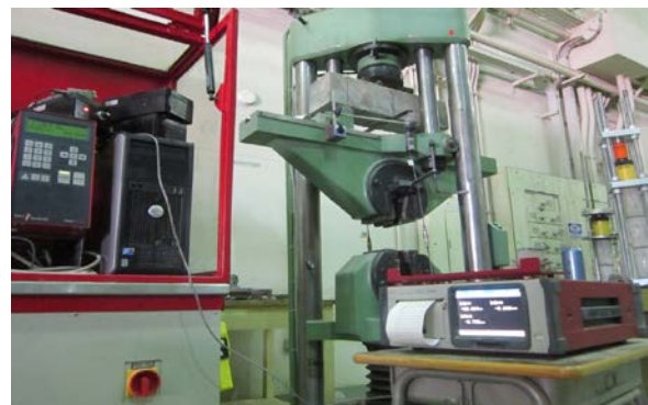
Fig. 3 : Flexural characteristics testing setup.
