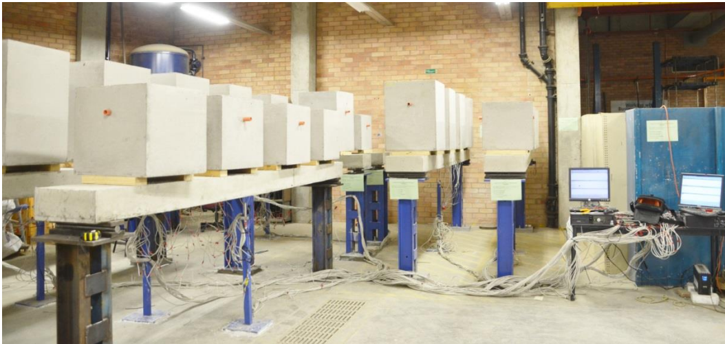
Figure 3. General view of flexural long-term tests under load.
