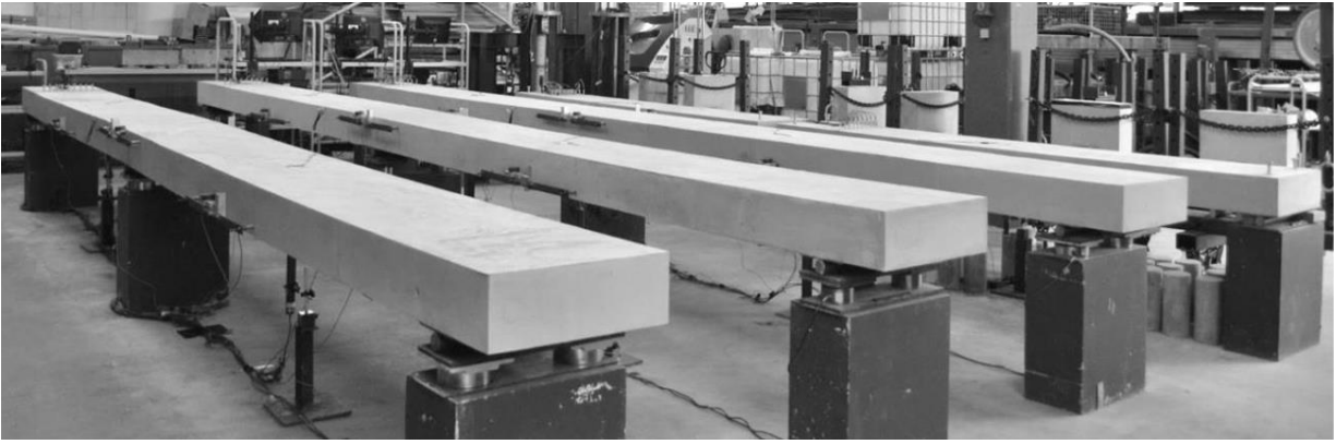
Figure 5. Reinforced concrete slabs subjected to only self-weight.
