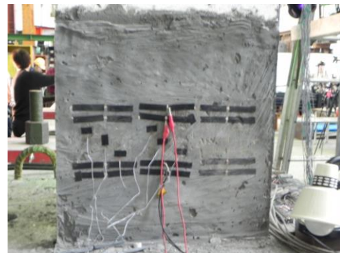
Figure 16. Test setup of CFRC for strain measurement.
