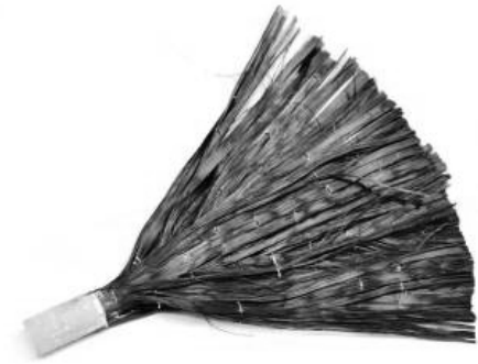
(b) Hand-made FRP anchor
