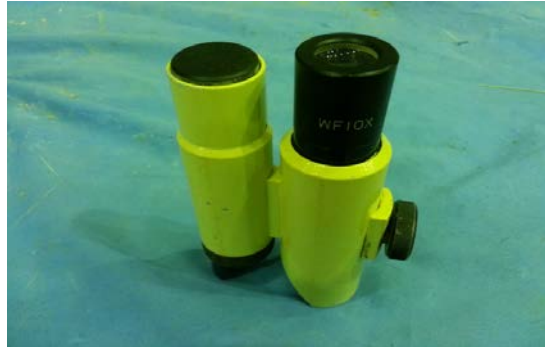
Fig. 4 : The microscope used for measuring crack width.
