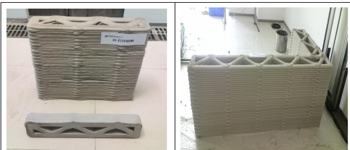
Figure 3.6 3D printing construction members
