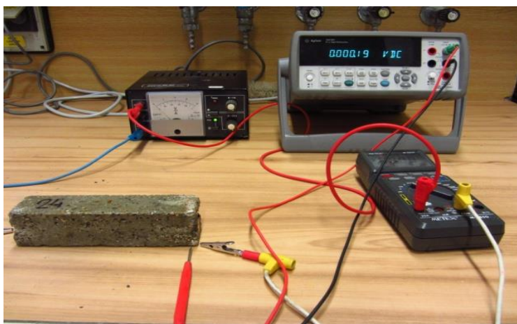
Figure 7. Set for measuring with Ohm method
