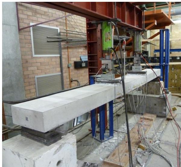
Figure 2. Short-term flexural test arrangement for all specimens.
