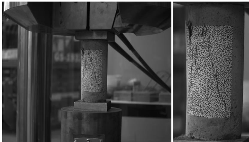
Figure 9. Failure mode of small cylinders
