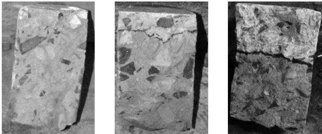
Figure 7 Example colourimetric test specimens showing increasing depth of chloride ion penetration from left (no white precipitate, all brown i.e. no colour change border) to right.
