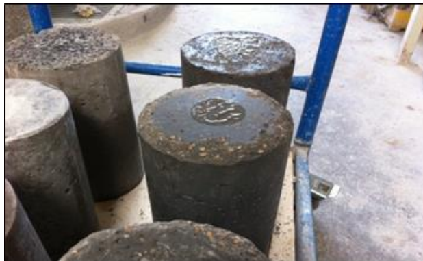
Figure 13. Recipe 1 (100% PFA) after 420 freeze-thaw cycles.
