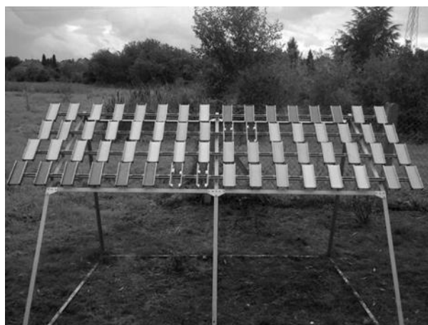
Figure 2. In-Situ bench for the colonization of mortars
