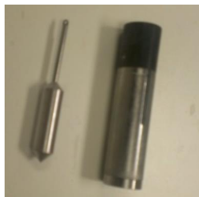
Figure 3. (left) Rheometer, (right) inner and outer cylinder.
