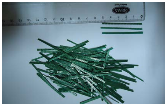
Fig. 1 : Picture of 50 mm long RP fibres used in the study.
