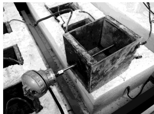
(b) Modified mould for temperature measurements
