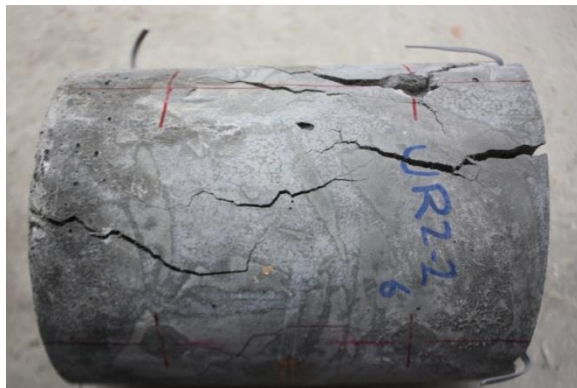
d) specimens having three stirrups 3φ6 (1.7%)
