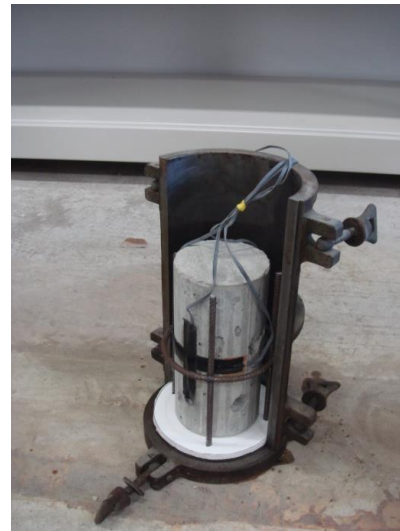
Specimen Type 1 (consist of strain gauges on the core surface) Stirrup: 1 \phi 6 (0.56%)
