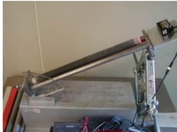
Photo 2. Length change measuring device
