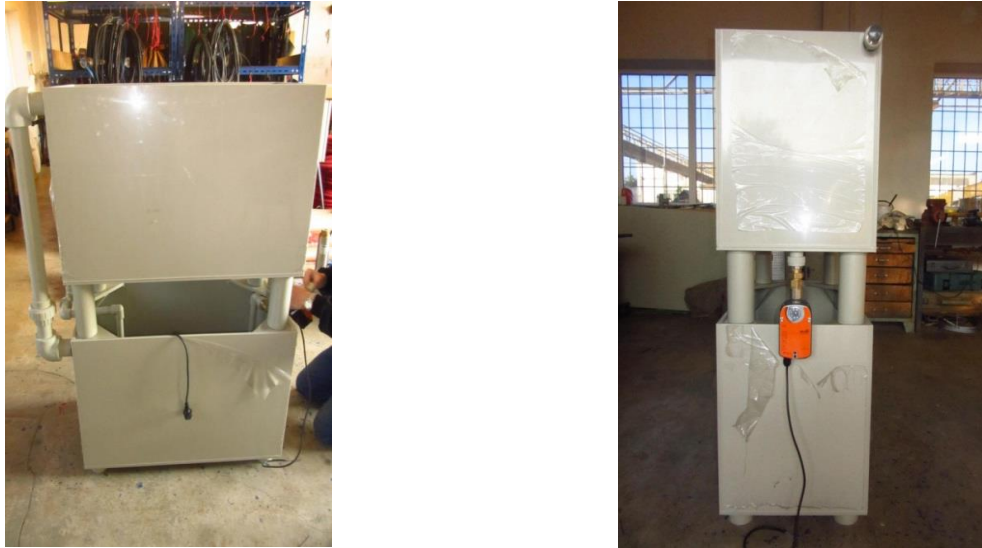
Figure 6. Apparatus for accelerated process of degradation of test specimens
