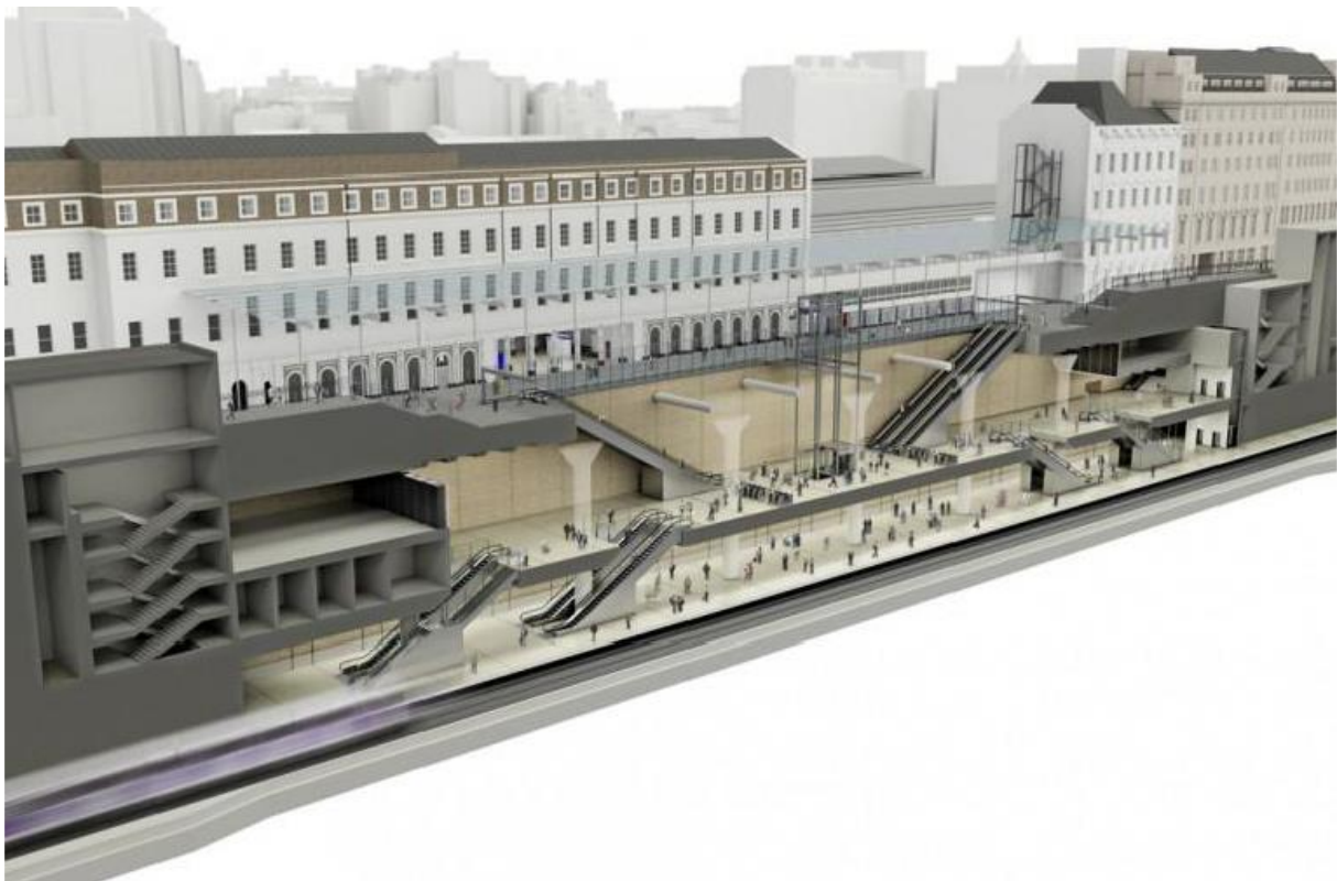
Figure 1: Architect's section through new station
