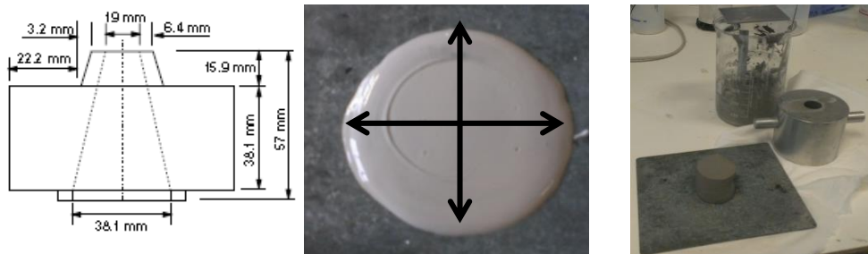
Figure 1. (left) Mini-slump cone dimensions, (middle and right) Test in action.
