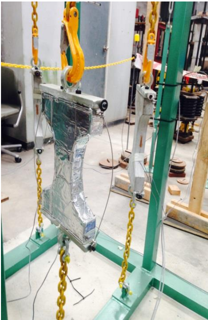
Figure 8 Specimen wrapped in self-adhesive foil to eliminate drying.
