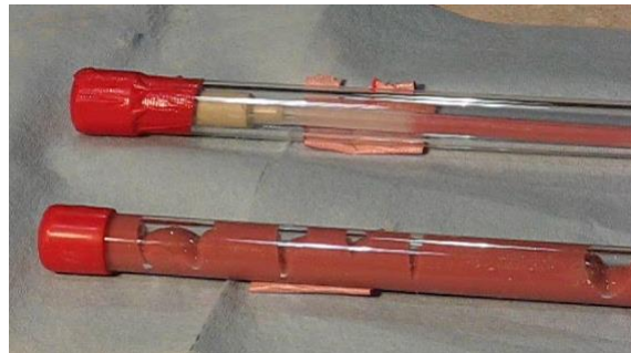
Figure 12. Voids in injection
