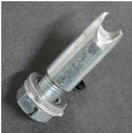
Figure 1. Ferrule that fractured during installation (source: [7]).
