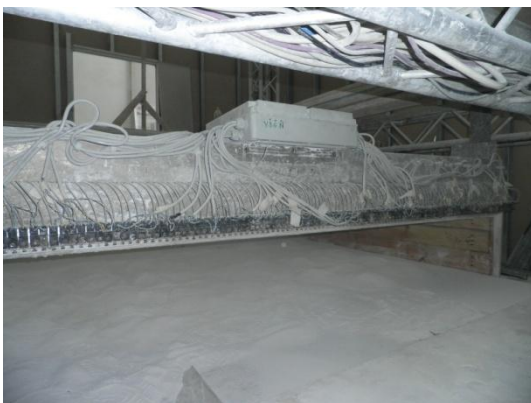
Figure1: 3D-shape prototype printer and printed object using Sorel cement (photos by A. Palomo)
