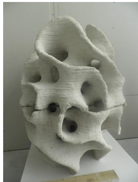
Figure1: 3D-shape prototype printer and printed object using Sorel cement (photos by A. Palomo)
