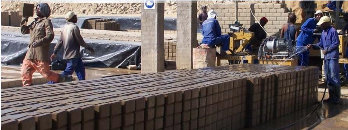
Figure 8: The blocks are wetted and then covered with a dark plastic sheeting.
