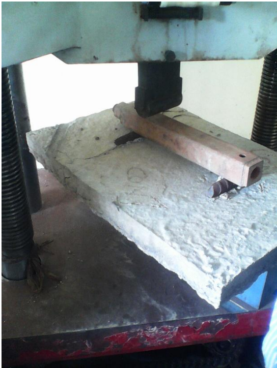
Figure 1: Flexural strength test
